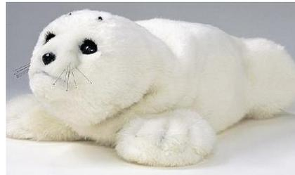
**Figure 2. PARO robot - a seal shaped therapeutic robot**
